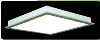
Room Size: 18 X 20 feet, Indirect T8 Fluorescent Luminaires 5 X 72W = 360W with an Average Illumination of 125 LUX Replaced with 25nos 1'x1' 6W Troffer Lights 25 X 6W = 150W Obtaining Average Illumination of 180 LUX
