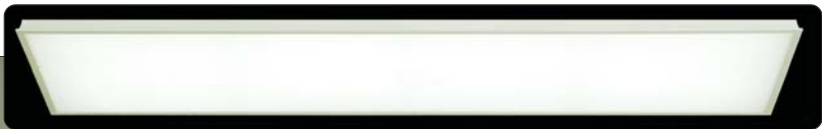
Room Size: 20 X 28 feet Indirect T8 Fluorescent Luminaires 6 X 72W = 432W with an Average Illumination of 150 LUX Replaced with 6nos 1' X 4' 24W Troffer Lights 6 X 24W = 144W Obtaining Average Illumination of 150 LUX
