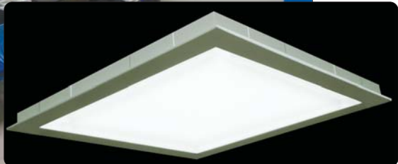
Room Size: 10 X 10 feet Indirect 2' X 2' CFL Luminaires 2 X 36W = 72W with an Average Illumination of 100 LUX Replaced with 2' X 2' 40W Troffer Light Obtaining Average Illumination of 200 LUX
